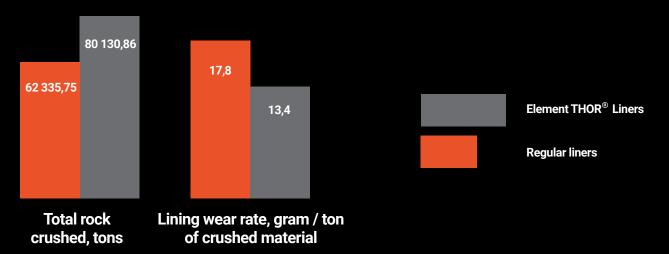
\* Based on trials of 6 sets of THOR<sup>®</sup> cone medium coarse crusher liners in 2019.
